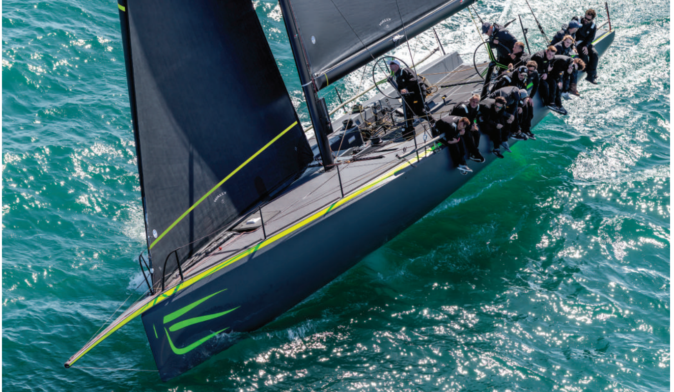
The wallyrocket51 has pedestal grinders and 15 crew in IRC mode; electric winches and a crew of 11 for one-design racing
